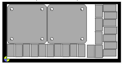
Nesting can be done manually, where parts are added to the plate one at a time. A part or group of parts can also be arrayed onto a nest. Nesting can also be done automatically.
